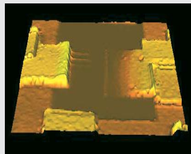
Fig. 1: Confocal picture of a chess board with 2 microns of period recorded in reflection mode.
